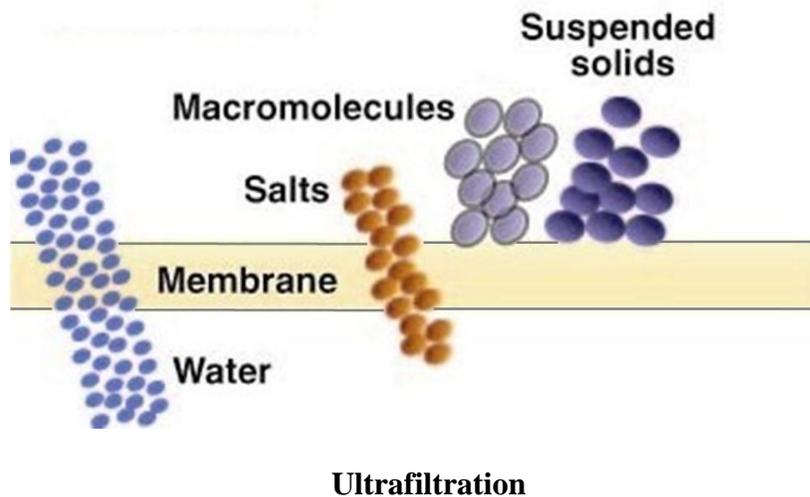
The above processes (MF and UF) separate contaminants based on a “sieving” process; that is, any contaminant too large to pass through the pore is rejected and exits in the concentrate stream.
