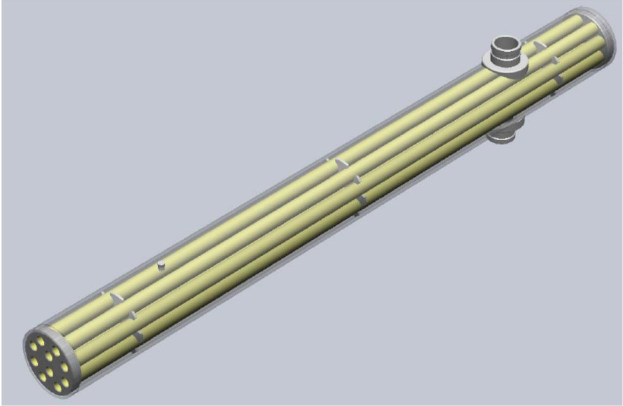
Each membrane module consists of ten 72" long tubes enclosed inside a PVC housing. Specifications on the modules and tubes are as follows:
