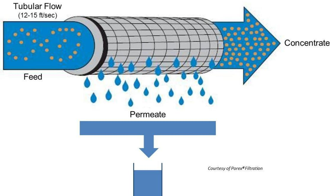
Specifically, the tubes are 1" I.D., with a polyethylene substrate supporting a PVDF (polyvinylidene fluoride) layer with 0.10 $\mu$  pores. The membrane modules are illustrated below.
