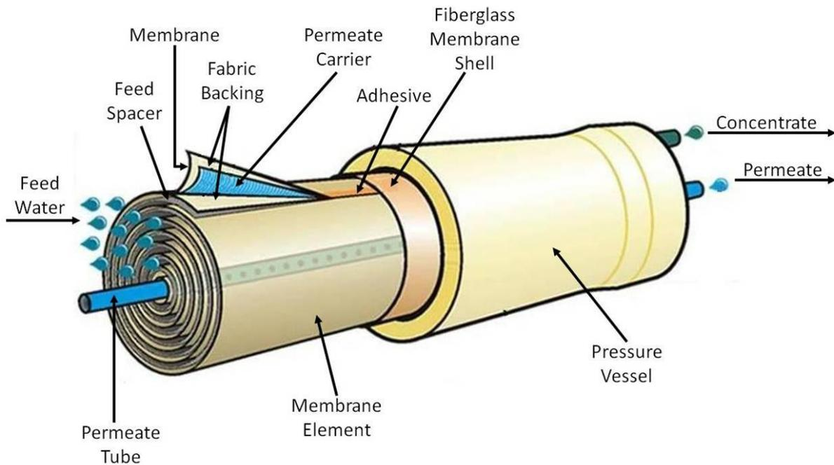
Although the least expensive of all the membrane element configurations, spiral wound reverse osmosis membrane elements are the most susceptible to fouling by suspended solids. In many cases, the normal multimedia filtration process, often utilized in lime softening, does not provide sufficient suspended solids removal to minimize downstream membrane fouling. This is where the superior filtration capabilities of MF technology can be exploited.
